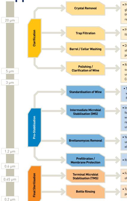
• Potassium bitartrate and calcium tartrate crystals are naturally occurring precipitates in wine which form non-hazardous glass like crystals. These crystals are undesirable and need to be removed during production. To remove the crystals the wine is chilled to just above freezing point, facilitating crystallisation and precipitation and the crystals can then be removed by centrifuge and filtration or filtration alone.
